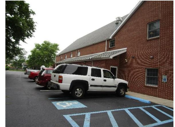
Pervious pavement can be installed along the southeast end of the parking lot to capture runoff from the disconnected downspouts along the east side of the building. Pervious pavement allows water to infiltrate through the surface. A preliminary soil assessment suggests that more soil testing would be required before determining the soil's suitability for green infrastructure.
